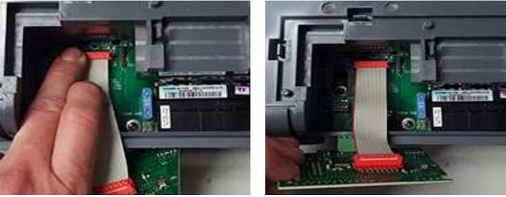
The interface board is held in place by three plastic clips on the housing.
