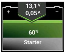
The bar height of the battery indicates the level of the battery. The lower grey portion of the battery is the unusable portion of the battery's nominal capacity that was determined at the last complete discharge. This portion provides information about the battery's state of life.
