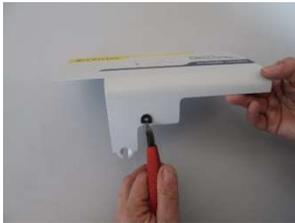
Inserting the rubber cable grommet
