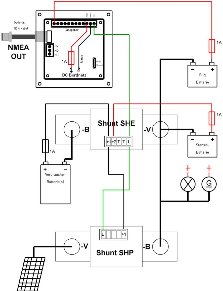
The LIN bus connection between the monitor and the shunt is made via a 1-wire cable. This can also be any or an existing cable. For mechanical reasons, the cable cross-section should be min. 1mm<sup>2</sup> and max. 1.5 mm<sup>2</sup>.
